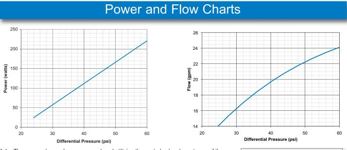
Note: The curves shown above were produced utilizing the control valve downstream of the generation unit. For detailed power and flow calculations, please contact the factory at 800.942.6326 or the sales agent nearest you to perform an analysis using our Cla-Power® Software.
